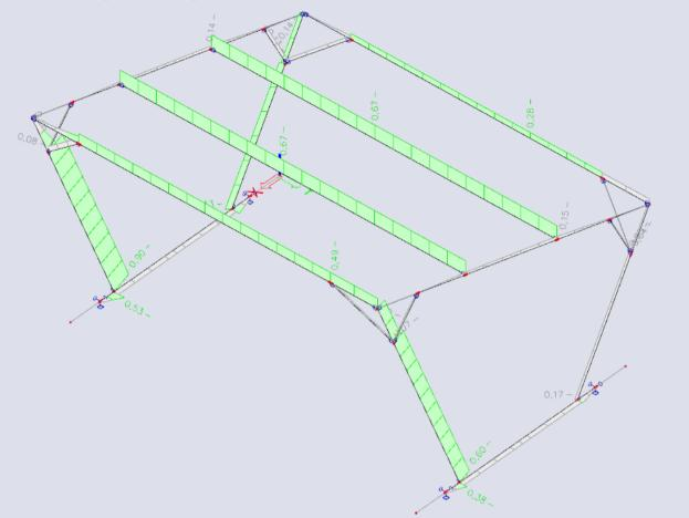
As can be seen from the image, the sections of front corner posts can achieve the usage of 90%. This is due to stability check. Section check usage is only about 50% of the section's strength so there is no risk of the post losing its load capacity. Stability is the determining factor because the posts are cantilevered.
