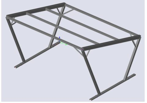
All connections between elements are hinged, allowing rotations, except for the connection between corner post and base rail, where rotations along the length of the base rail are not allowed.
