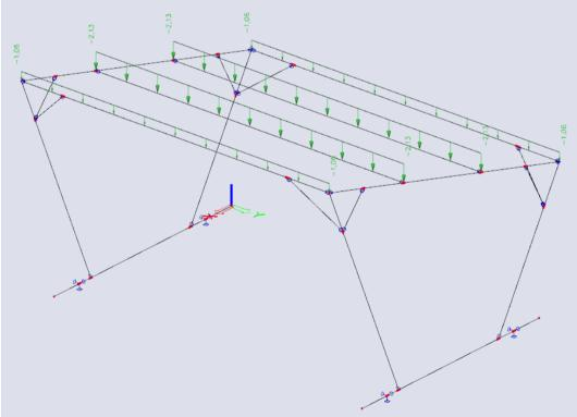
Wind load on roof (downward) applied:
