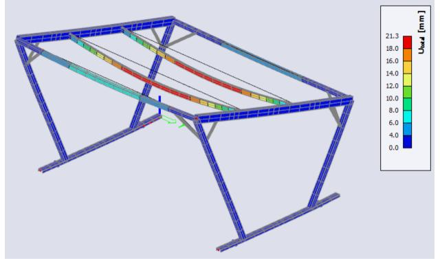
Maximum vertical displacement of roof purlins (SLS 1):
