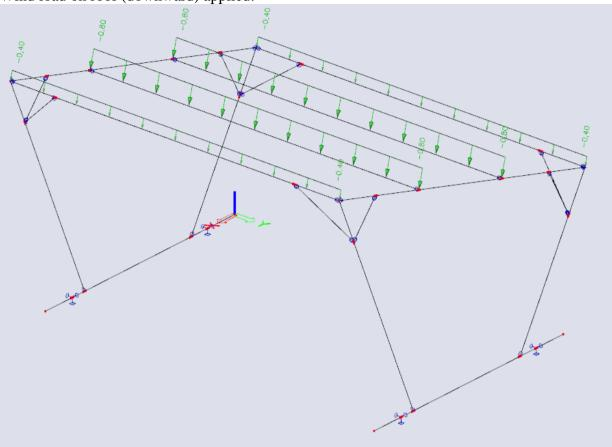
Wind load on roof (upward) applied:
