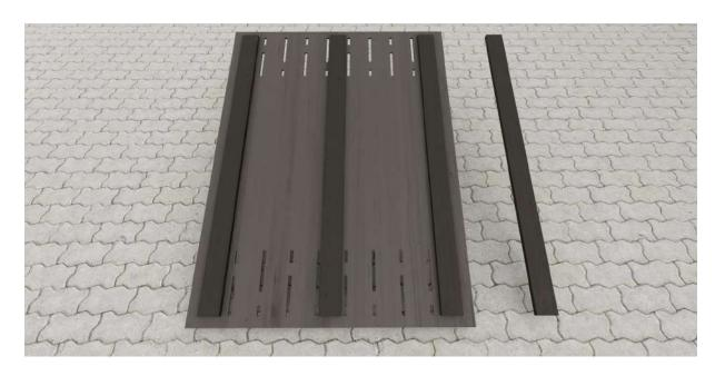
O Step 27 - Connect plywood ceiling onto purlins with screws
