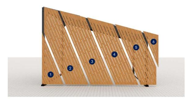
O Step 21 - Connect mortise and tenon joints and install the next row of CLT panels
