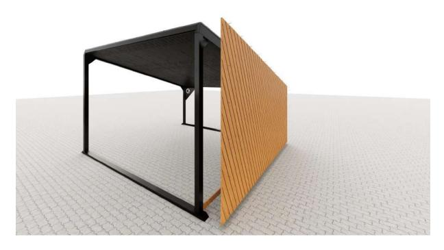
O Step 23 - Connect timber board behind CLT timber cladding's lower edge with screws
