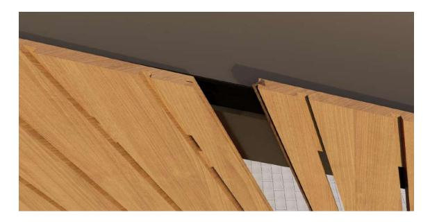
O Step 23 - Connect all CLT panels with screws
