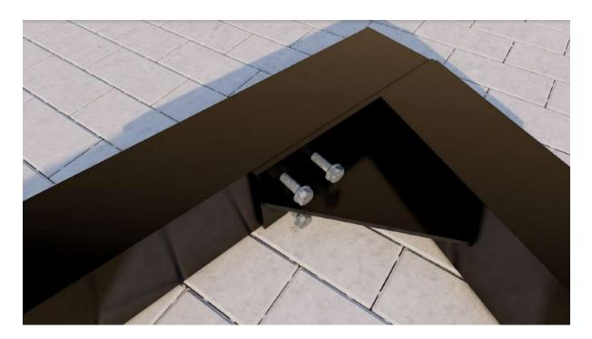
O Step 8 - Lift up both sides of carport and connect eave strut
