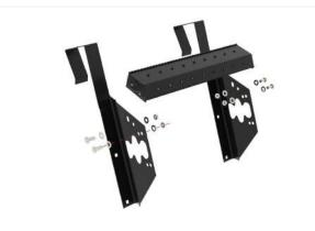
**Step 3:** Brackets can be attached together with M8x20 bolts, nuts and washers that are equipped with the system. Note that brackets are connected with round head square neck bolts.
