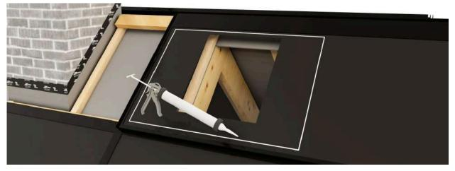
• Add the bottom cover of the roof access hatch.
