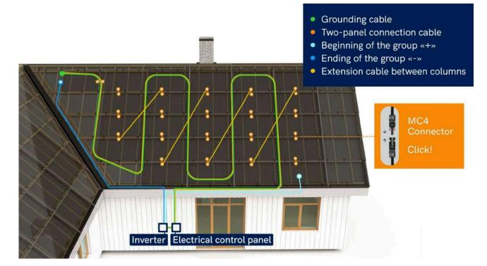
• Bring the earth wire down to the ground. Make sure that the grounding wire is safely apart from objects that may harm the cable and its functionality.
