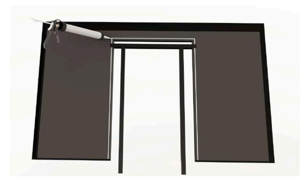
• Once the frame is sealed with silicone, attach it to the dummy panel using screws.
