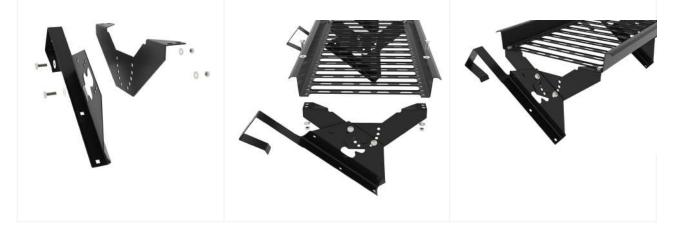
• Step 1: Start hook and walkway brackets should be fastened together on the ground. Then, fasten the hooks to the battens using 8 x 50 screws.
