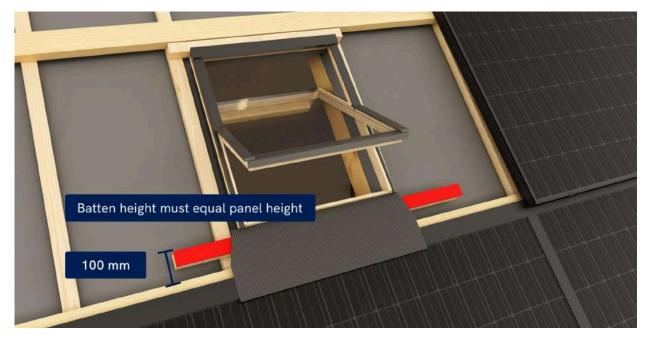
• If the dummy panel is cut, start by applying silicone to seal the roof window and the frame of the dummy panel.
