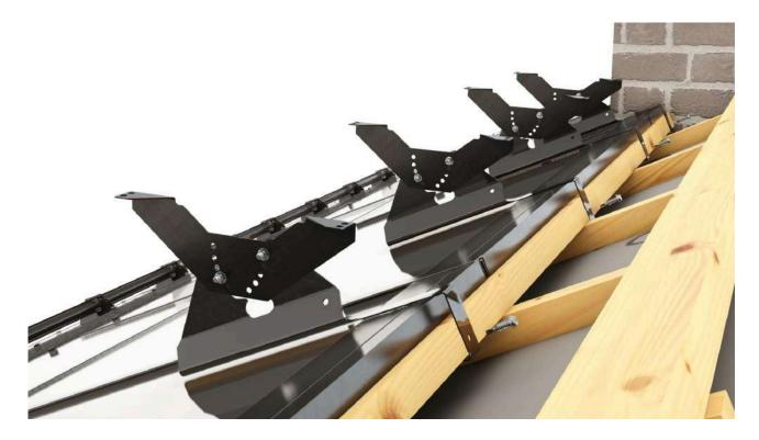
• Step 2: Add walkway on top of the brackets and fasten it with M8x20 bolts nuts and washers.
