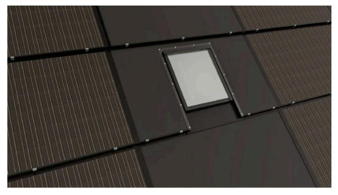
**Disclaimer:** The bottom roof window flashing must extend to another PV module. It should not lay between battens or be positioned on battens.
