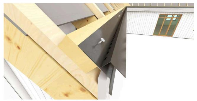
• The panel and the gutter must be aligned correctly to ensure that water does not run over the gutter. Proper placement guidelines can be found in the gutter installation manual.
